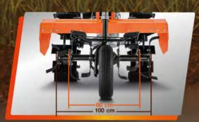
80 cm width rotary can be extended up to 100 cm with the extension shaft\* to deliver working capacity of 0.45-0.50 Acre/hr (1.14-1.26 rai/hr)\*\* and can work close to the field border, allowing for more planting space.
